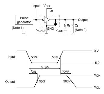
Note 1: Pulse width 50  $\mu$ s, Duty cycle 10% Output impedance 50  $\Omega$ , tr ≤ 5 ns, tf ≤ 10 ns
