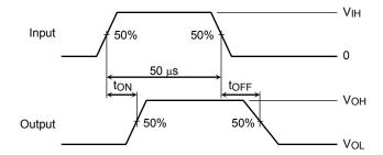
Note 1: Pulse width 50 μs, Duty cycle 10%
