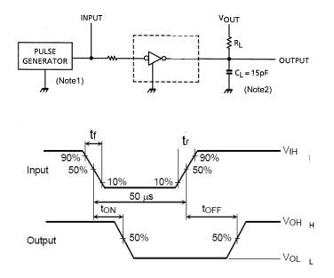
Note1: Pulse width 50  $\mu s,$  Duty cycle 10 % Output impedance 50  $\Omega,$  tr  $\leq$  5 ns, tf  $\leq$  10 ns, V\_{IH} = 5.0 V
