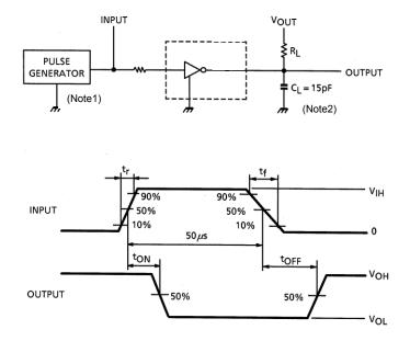
Note1: Pulse width 50  $\mu$ s, Duty cycle 10 % Output impedance 50  $\Omega$ , tr ≤ 5 ns, tf ≤ 10 ns, V<sub>IH</sub> = 5.0 V
