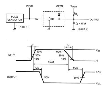
Note 1: Pulse width 50  $\mu$ s, Duty cycle 10% Output impedance 50  $\Omega$ , tr  $\leq$  5 ns, tf  $\leq$  10 ns, VIH = 5.0 V
